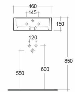
Dimensions: All dimensions in mm tolerance ±5% for below 200mm and ±3% for above 200mm.
