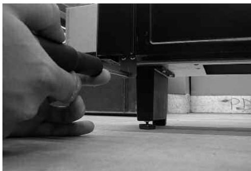
Fig. 8 Removing the Lower Outer Case Fixing Screws
