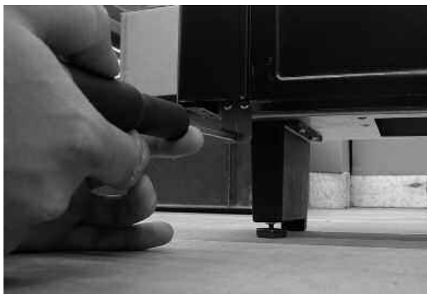
Fig. 3 To Remove the Lower Outer Case Fixing Screws
