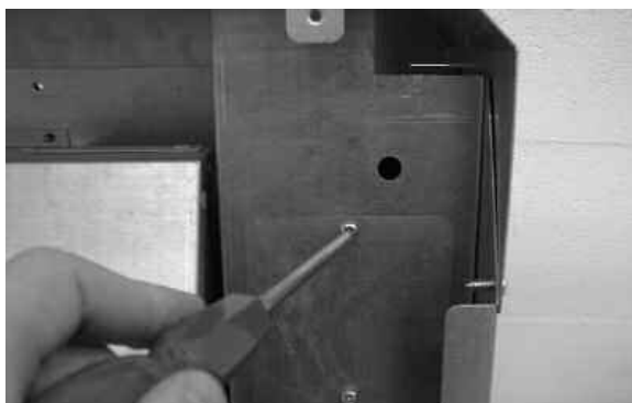
Fig. 12 Control Valve Panel Removal
