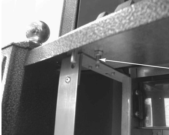
Front bezel retaining screws (1 off each side)
