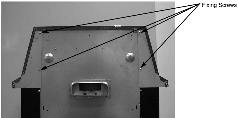
Fig. 6 Removing the four canopy rear fixing screws
