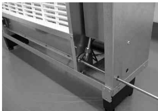
Fig. 11 Injector fixing bracket removal
