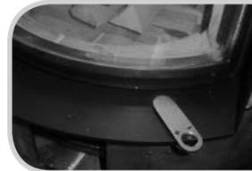
If the furnace is rotated back to its normal position, the air control lever has to be turned by hand to the left to the „+“ position in order to allow the fire to ignite with sufficient combustion air. The combustion air supply is then completely opened.
