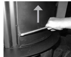
The firing door can be locked for a short time for cleaning purposes. For this purpose, push the locking mechanism (which is located on the bottom right when the firebox door is tilted) towards the bolt and connect it. To close the door, open this slightly more than the current 90°. The lock is released and the door can be closed.
