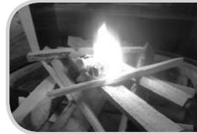
Light the pyre, close the fire door, and turn the firebox by means of the control handle (using the heat-resistant glove) counter-clockwise back to the normal position.
